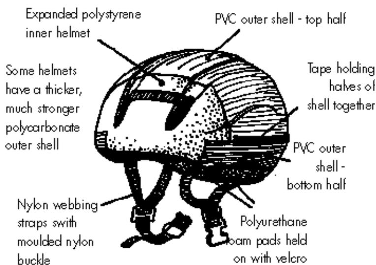
Figure 11 Cut away, labelled diagram of a safety helmet to show the materials used to make it.
