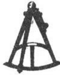
Information from stars An octant measures the altitudes of stars. It was used to find the bearing of a ship or the time as night.
